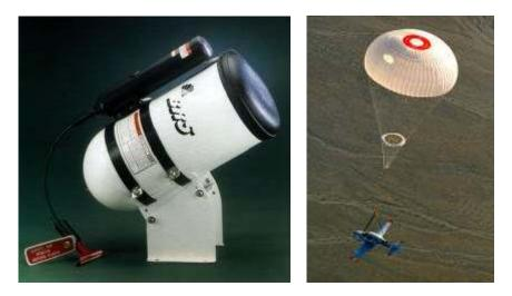
Ballistic Parachute Systems have an actuation T-handle (usually red) within reach of the pilot attached to a sheathed cable. The cable runs directly into the rocket igniter attached to the parachute container. In most cases, the parachute deploys up and aft, and the entire assembly is located close to the aircraft center of gravity; around where the wing and fuselage meet.
